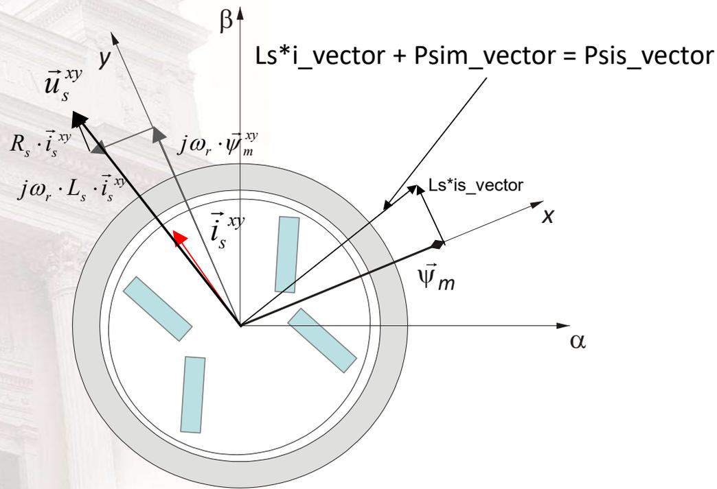
$$\vec{u}_s^{xy} = R_s \cdot \vec{i}_s^{xy} + L_s \cdot \frac{d\vec{i}_s^{xy}}{dt} + j\omega_r \cdot \overbrace{(\vec{\psi}_m^{xy} + L_s \cdot \vec{i}_s^{xy})}^{\text{Psis\_vector}}$$
