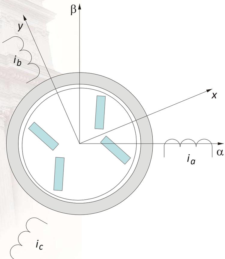
$$\begin{aligned} & \sqrt{\frac{2}{3}} \left( u_{sa} = R_s \cdot i_{sa} + \frac{d\psi_{sa}}{dt} \right) \\ & + \sqrt{\frac{2}{3}} \cdot e^{j\frac{2\pi}{3}} \cdot \left( u_{sb} = R_s \cdot i_{sb} + \frac{d\psi_{sb}}{dt} \right) \\ & + \sqrt{\frac{2}{3}} \cdot e^{j\frac{4\pi}{3}} \cdot \left( u_{sc} = R_s \cdot i_{sc} + \frac{d\psi_{sc}}{dt} \right) \\ \hline \vec{u}_s &= R_s \cdot \vec{i}_s + \frac{d\vec{\psi}_s}{dt} \end{aligned}$$
