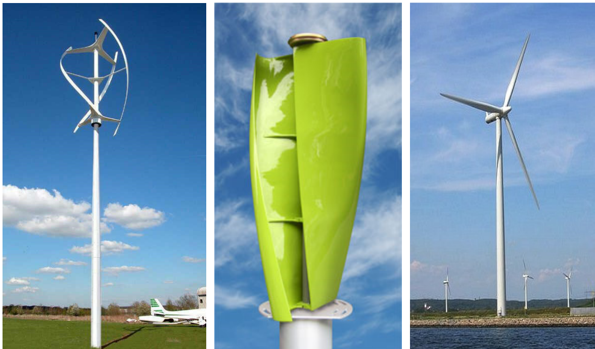
Figure 1. From left: three blades VAWT, Savonius VAWT and conventional HAWT
