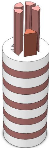
**Figure 15 Showing model of male connector using new BalSeal concept**
