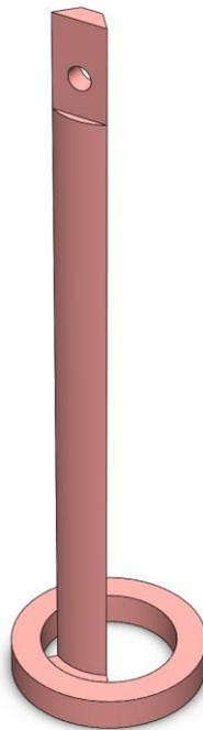
**Figure 17 Illustration of phase ring brazed to copper bar**
