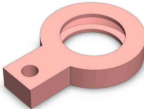
**Figure 23 Illustration of female phase-ring brazed to the block connecting to cable**
