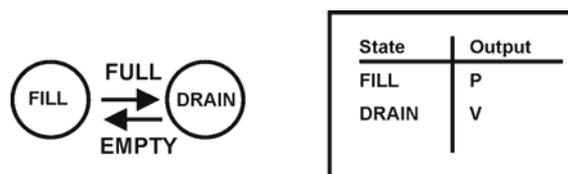
To implement this in ladder directly is not possible with our normal method. Since the state transition is made safe by breaking/leaving a state upon the arrival to the next state a problem occurs. If the next and the previous states are the same state it means that the entry condition and the exit condition will contain the same state but in invers in the exit-part. A signal and it's invers in series can never be true.
