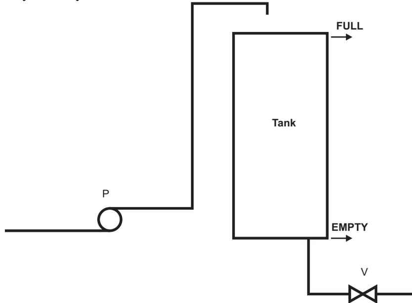
Draw a minimal state graph for the control of this system and write an output signal table. Explain why this graph can't be directly implemented in a ladder program. Make the necessary modifications and write a working ladder program for the control.
