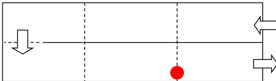
Figure 6-4 Layout of the aeration basin at Himmerfjärden WWTP. The dot indicates the position of the oxygen sensor.
