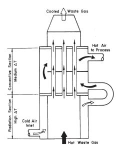
Figure 3.5: Combined radiation and convection recuperator (Turner & Doty, 2007).
