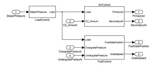
Figure 5.3: Block diagram of the overall control system.
