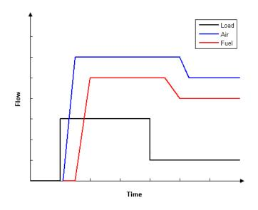
Figure 3.1: Cross-limiting of air and fuel signals.
