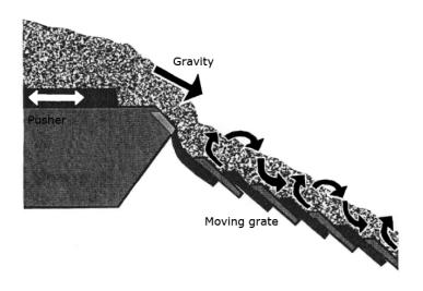
Figure 4.3: Principle of grate movement (MARTIN GmbH, 2008b).
