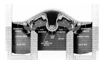
Figure 2.4: Cross-section of an underfeed stoker (Oland, 2002).
