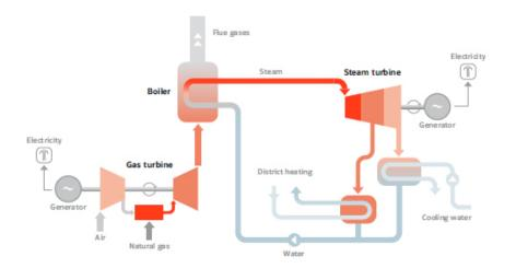
Figure 4.4: The principal operation of the Öresundsverket power plant (E.ON, 2010).
