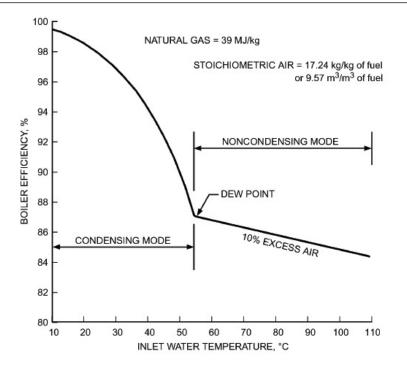
Figure 2.3: The effect of inlet water temperature on efficiency (ASHRAE, 2008).
