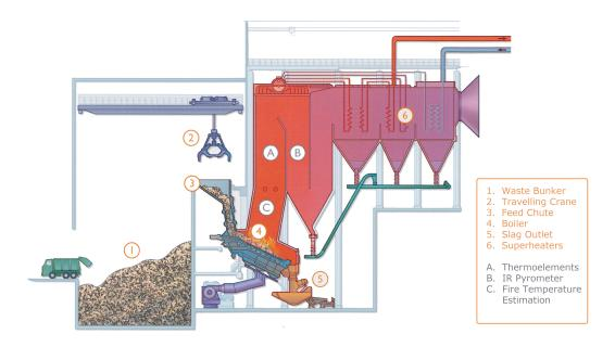
Figure 4.2: Illustration of Boiler 4 at Sysav (Sysav, 2010a)
