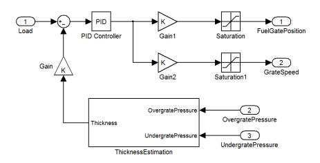
Figure 5.6: Block diagram of the fuel control system.
