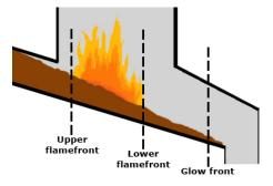
Figure 3.4: Illustration of the flame fronts and the glow front.
