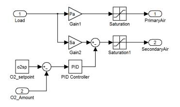
Figure 5.5: Block diagram of the air control system.
