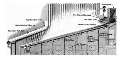
Figure 2.5: Cross-section of an overfeed massfeed stoker (Oland, 2002).
