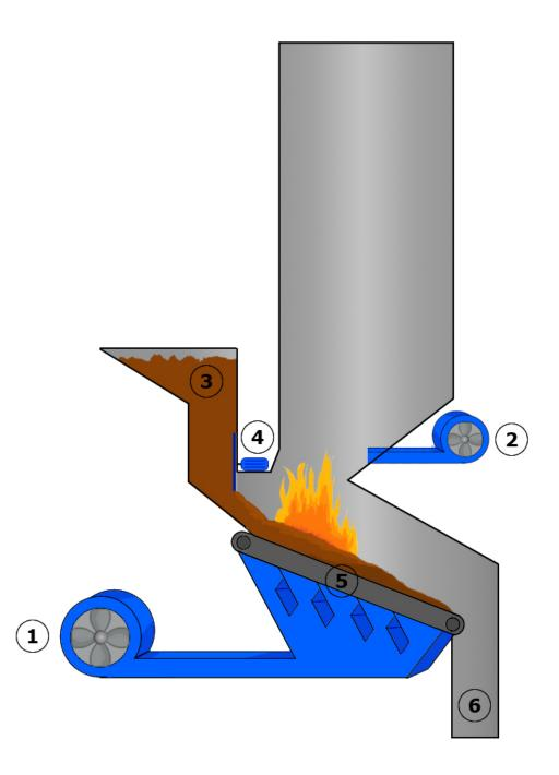
Figure 5.1: A cross-section of the simulated boiler system. The labels are explained in the text.
