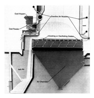
Figure 2.6: Cross-section of an overfeed spreader stoker (Oland, 2002).
