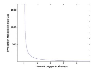
Figure 3.3: Hypothetical  $CO-O_2$  characteristic curve.
