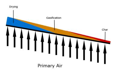
Figure 3.2: Combustion bed.
