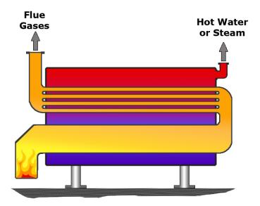
Figure 2.1: A two-pass firetube boiler.
