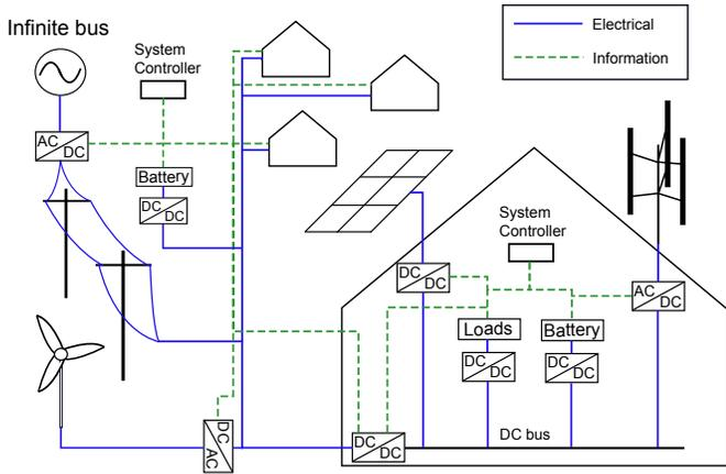
Fig. 1: Schematic figure over a smart house connected to a smart grid
