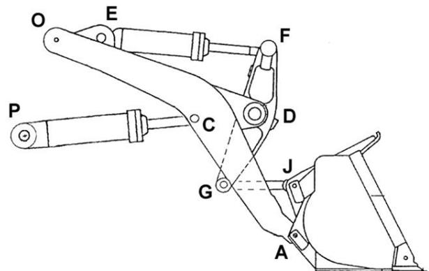
Figure 2 Z-linkage, the most used linkage. [2]
