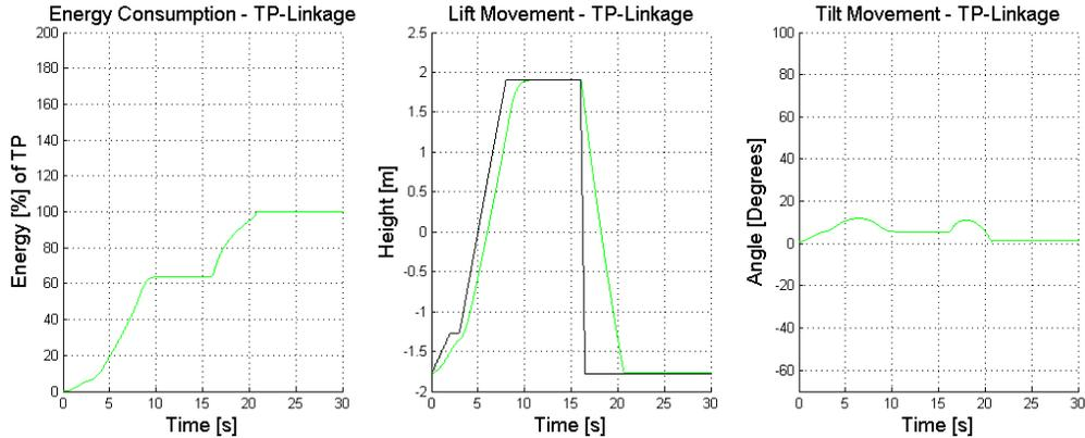
Figure 3 Simulation results of lifting and lowering the TP-linkage. Black curve is reference height and green curves are the results from simulations.
