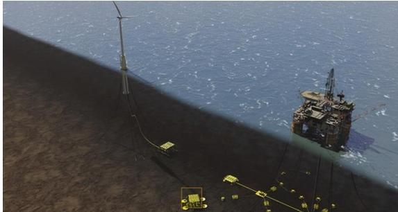
Figure 3. Floating wind power can be used to power the water injection pump raising the pressure of the oil reservoir and thereby increasing the potential oil extraction. Such an application could dramatically reduce the CO<sub>2</sub> emissions of offshore oil & gas activities on the Norwegian continental shelf.
