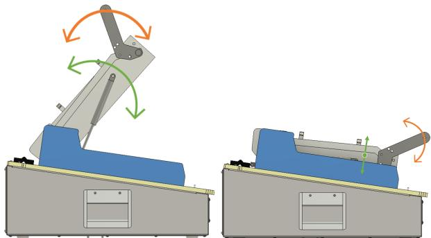
Figure 2: The left figure shows the opening/closing and the right picture show the locking/unlocking.
