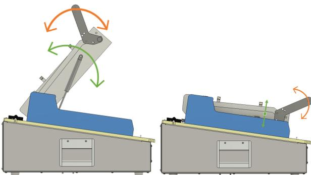
Figure 2: The left figure shows the opening/closing and the right picture show the locking/unlocking.
