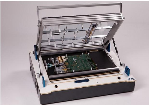
Figure 1: A typical FCT-fixture made by MG with a PCB placed inside.
